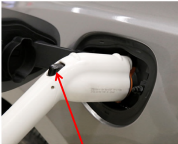
Press the EVSE Recharge Coupler button and pull to remove.
