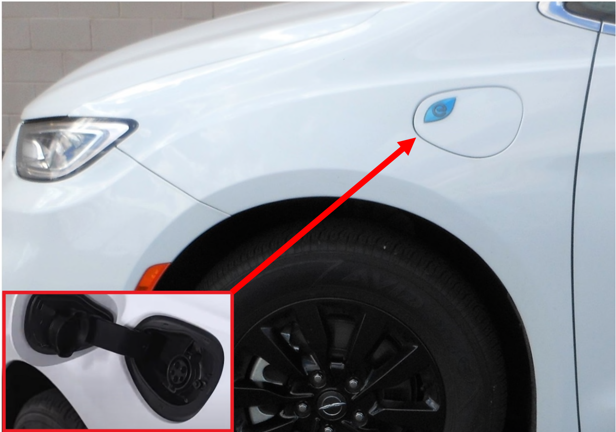
A charge port door with the “e” leaf logo, which is located at the driver-side fender panel.
